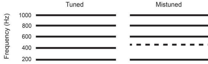
Figure 1. Structure of stimuli used in the current study. Harmonic complex tones consisted of 5 harmonics with a fundamental frequency of 200 Hz. Stimuli were either tuned (left) in which each harmonic was an integer multiple of the fundamental (200 Hz) or mistuned in which the second harmonic was mistuned upwards by either 2% (408 Hz) or 16% (464 Hz).
